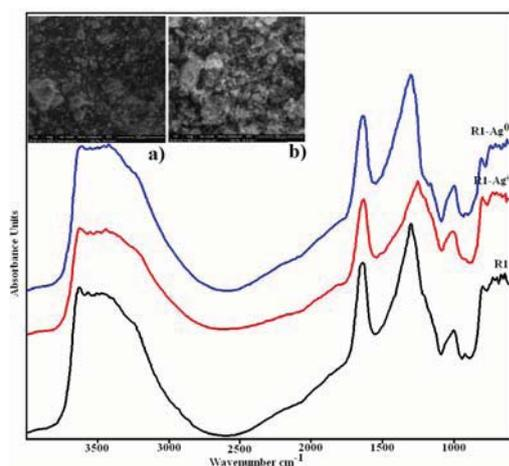
**Fig. 1.** FTIR spectrum of sample R1, R1-Ag and R1-Ag and SEM micrographs of R1-Na<sup>+</sup> (a) R1-Ag<sup>+</sup> (b)
